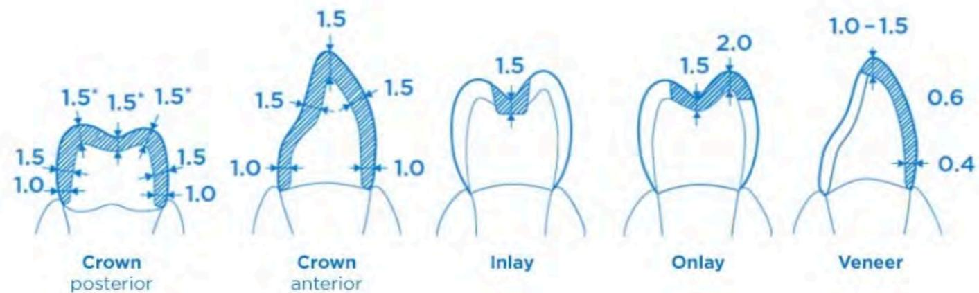
As with all CEREC restorations, the margins are the most critical part of the preparation and should be smooth and polished. Any milled restoration requires smooth polished margins so that the milling unit can adequately mill Celtra Duo (ZLS) restorations with ease.
